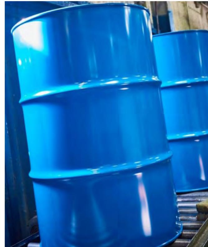
Increasing steel thickness can help prevent distortion. However, if the internal pressure buildup is so high the drum distorts, a vent should be considered. Vents can be used if they do not create a hazardous environment during transportation due to release of the contents. The same vendors that manufacture steel and fusible plugs can provide vented plugs.
