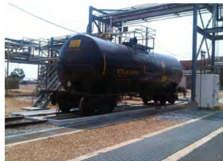
Figure 8. A railcar siding for unloading. Sidings may be adjacent to fixed storage tanks, in close proximity to the chemical process or located in a remote section of the facility.
