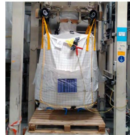
Figure 6. A Flexible Intermediate Bulk Container (FIBC) containing a dry solid chemical. Note the yellow lifting straps and the external grounding attachment.
