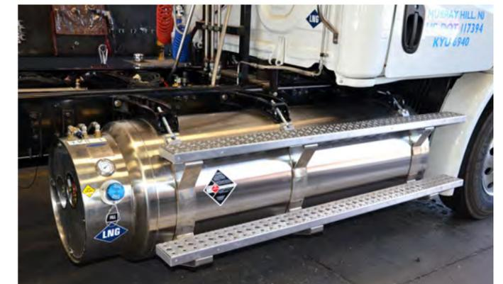
Truck fueled by LNG shows blue diamond placard near fuel tank.
