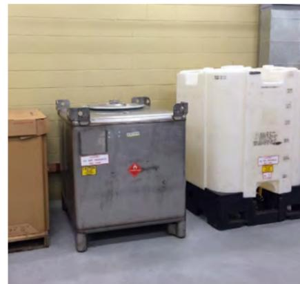
Figure 4. Examples of cardboard bag-in-box, metal, and plastic totes for transporting liquids.
