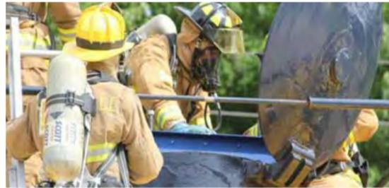
CSX Transportation "On Track" drill, 2010 - Asheville, North Carolina, Asheville Fire Department - "On Track" Drill applying a capping Midland kit to secure release from a defective valve. (Photo: Nick Ferroli, Compliance Associates)
