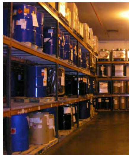
Figure 1. Bulk storage of chemicals in a warehouse in portable drums (steel, plastic, fiber) and metal totes. When needed, the chemicals are moved on pallets by hand truck or forklift to the chemical processing area.
