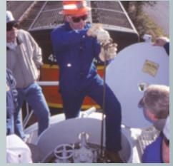
BNSF's Pat Brady demonstrates the fine points of a pressure tank car gaging rod. Through the use of air and water on the training cars, responders can better visualize what types of leaks they could be faced with.
